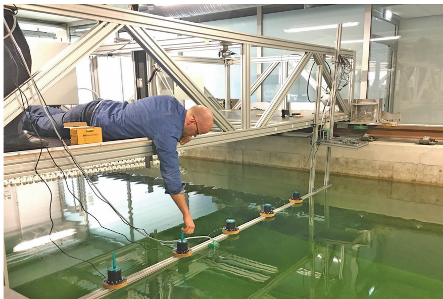
The 60m x 5m x 3m test basin at the SCC's Saaremaa facility enables users to analyse resistance and seakeeping behaviour
