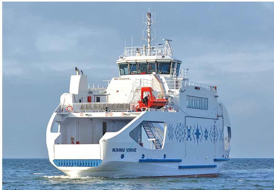
Kihnu Virve , one of the trio of 200-pax, 45m ice-breaking ferries built by Baltic Workboats for the Estonian Maritime Administration
