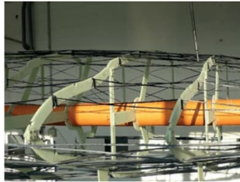
Production of inner structure of hull in strand laying process
